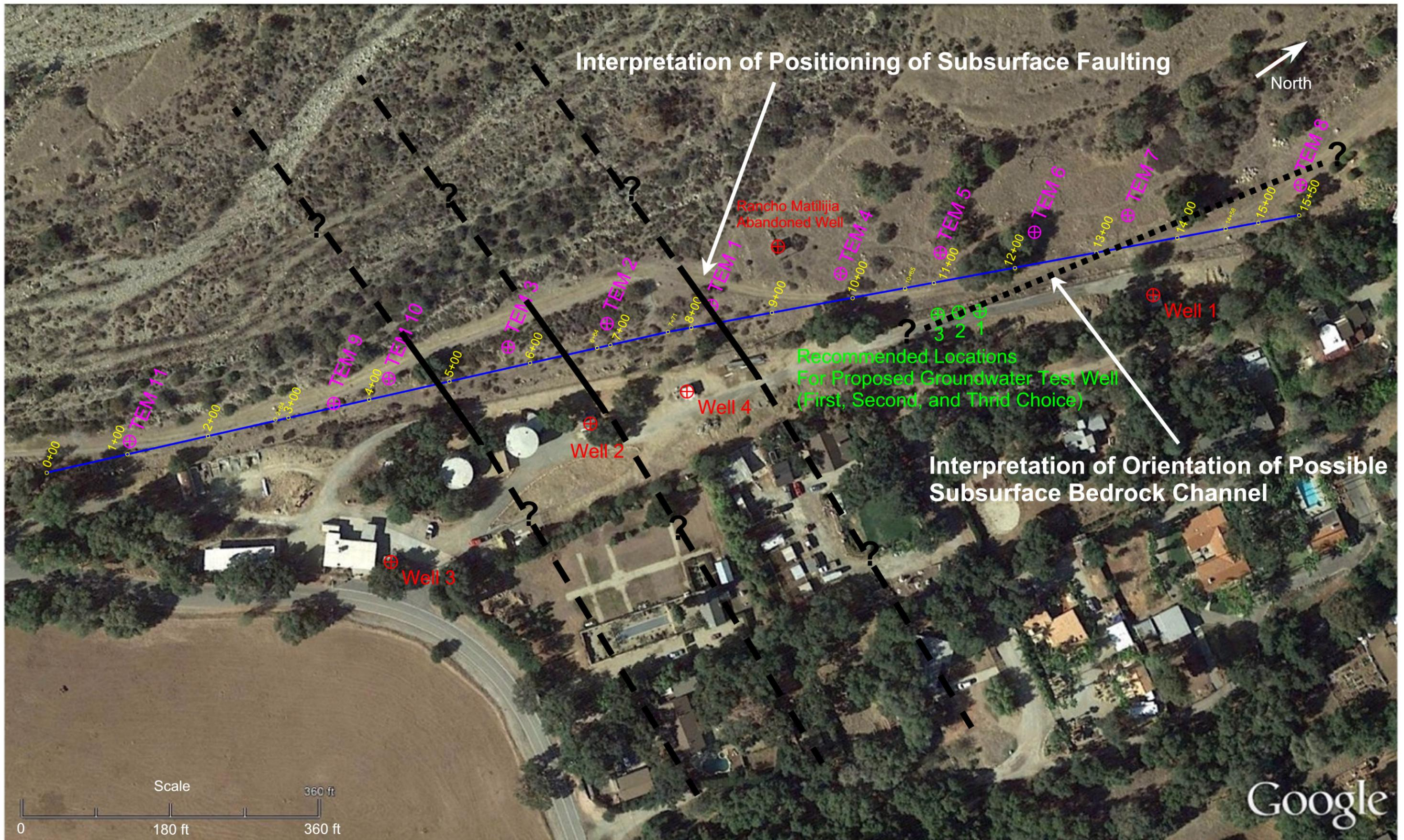
Site Map Showing Interpretation of Subsurface Faulting and Possible Bedrock Channel
