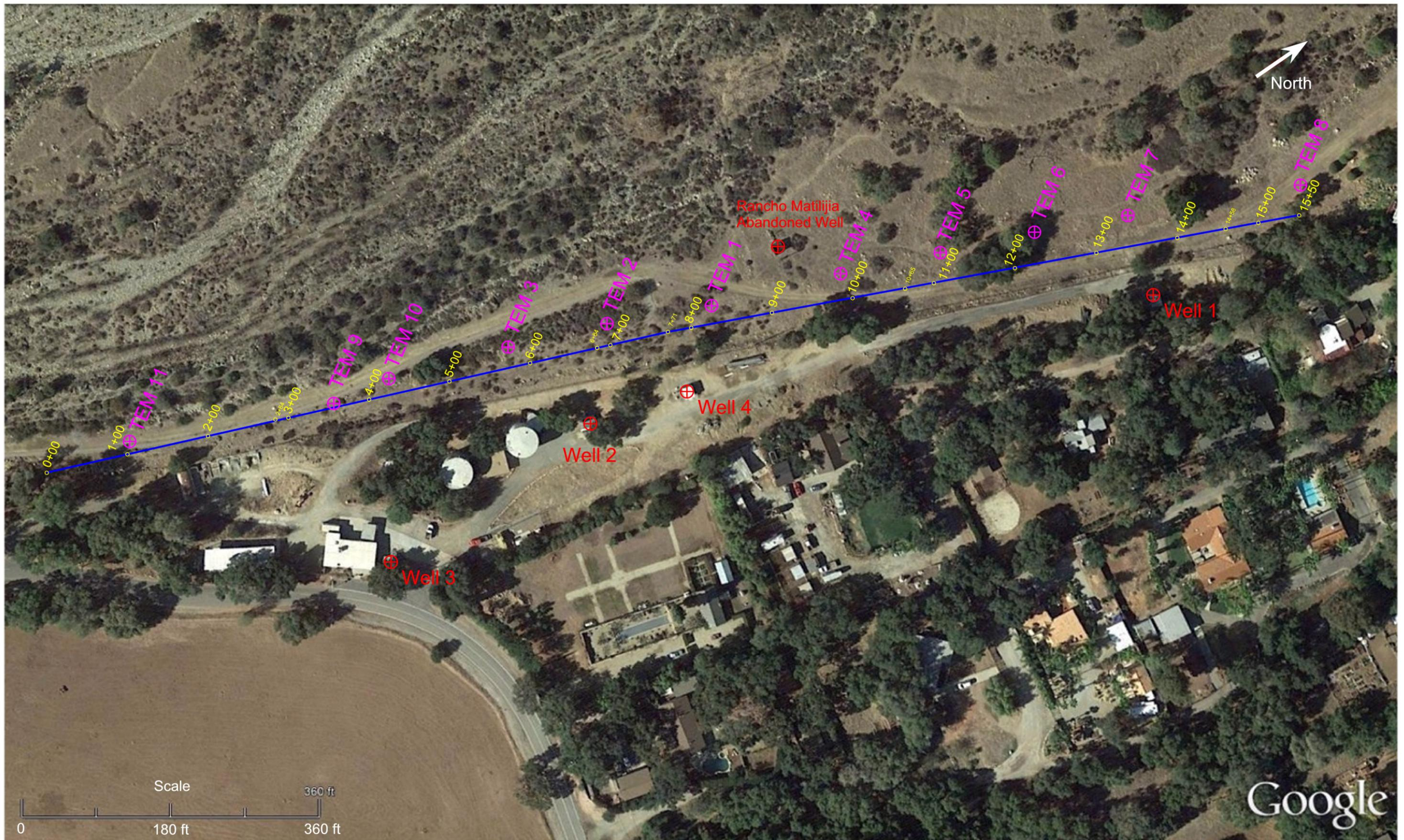
Site Map Showing Locations of Seismic Survey Line 1 and TEM Resistivity Soundings Ventura River Water District Facility Ojai, California
